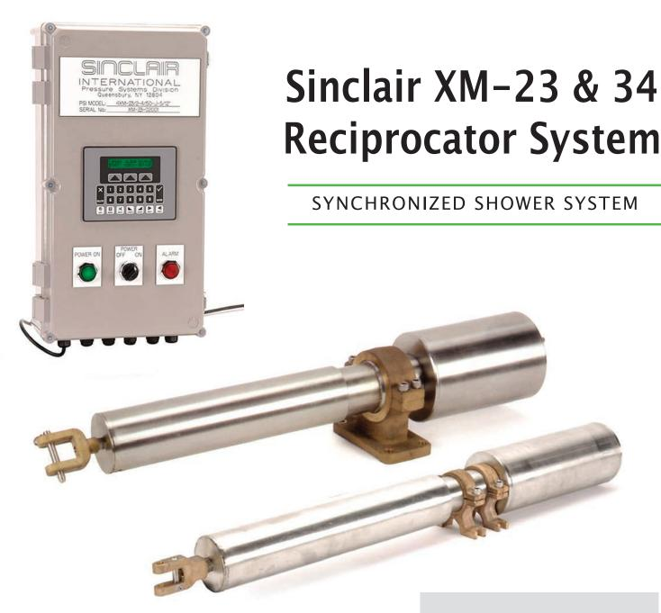
Sinclair's Model XM-23 & 34 are new systems for reciprocating showers on the paper machine, in which one (1) control panel can operate multiple drive units. All wetted parts are manufactured in either 316 stainless steel or anti-acid bronze, reflecting its intended use in paper mills
